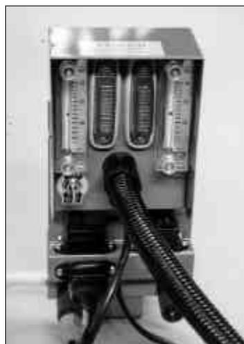
**If the ball drops** while operating **something is wrong** and the chemical is not being applied as required. If this happens while spraying **stop the unit** and rectify the problem before attempting to spray again.
