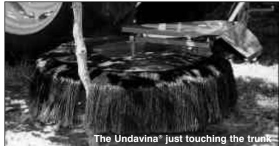
The trunk of the tree or vine should not be pushed more than 100mm (4") into the cover from its perimeter when passing. This will give a smooth operation and deflection and therefore extend the life of the machine.
