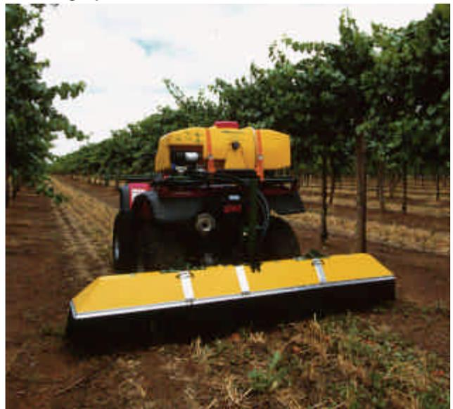
Spraymiser mounted to 4 wheel motorbike
